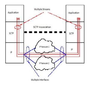
Fig 1: Schematic view of an SCTP association.
